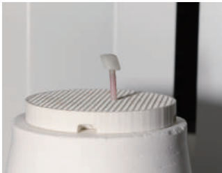
Put the sintering tray into the porcelain furnace and start sintering
